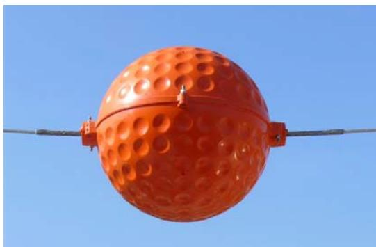
It is suitable for conventional earth wire and OPGW, and for phase conductor line. For the installation on OPGW it is required install first armour rods.
